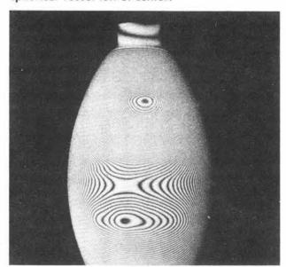
RESIDUAL DEFORMATION of a poor-quality vessel. The bullseye patterns represent local maximum deformations.
